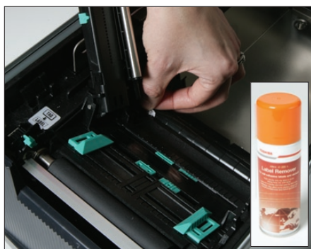
8. Remove any paper debris or label glue from the paper path, using the Label Remover if necessary (following the instructions carefully).
