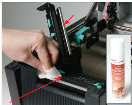
5. Spray some Platen Roller Cleaner on to a Toshiba Cleaning Cloth and gently wipe clean the platen and dumper roller.
